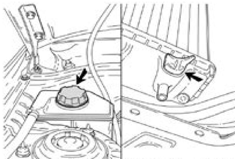
**Fig. 11- Removing Cap From Expansion Tank & Opening Radiator Drain Cock**
