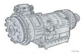
This service manual describes the design and function of the automatic gearbox. Powerbonic Generation III (produced from December 1995). The illustration above represents VT1706PT alternatively VT1906PT equipped with power take-off PTPT for the propositer shaft drive.
