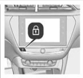
Press ft to lock. The LED in the button illuminates.
