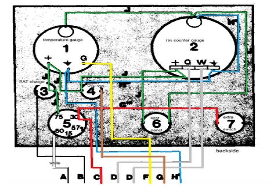
Volvo penta motor console wiring diagram (colour)
