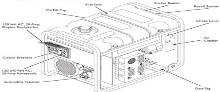
I 20 Volt AC, 20 Amp, Duplex Receptacles — May be used to supply electrical power for the operation of 120 Volt AC, 20 Amp, single phase, 60 Hz electrical, lighting, appliance, tool and motor loads.
