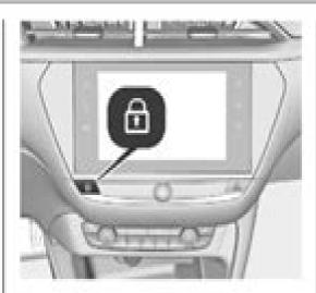
Press at to lock. The LED in the button illuminates.
