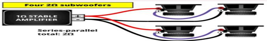
Result: OK BUT NOT GREAT - with a  $2\Omega$  total load the amp will be able to deliver good total power (not max. rated power) but each subwoofer gets ¼ of the total power output @  $2\Omega$ . (Ex.: for 500W @  $2\Omega$  each subw. can get 125W).
