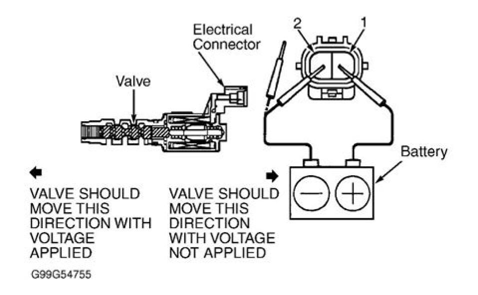
Fig. 13: Testing Oil Control Valve Courtesy of TOYOTA MOTOR SALES, U.S.A., INC.
