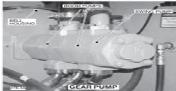
A gear pump consisting of three gear housing sections, all connected together internally supply hydraulic oil to all of the functions on the machine except the pilot system. The first two gear housings at the shaft end supply oil for the boom functions and the end gear housing supplies oil for the swing circuit.
