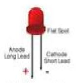
Connect LED as per the polarity
