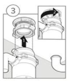
Twist and lock disposal onto sink mounting assembly
