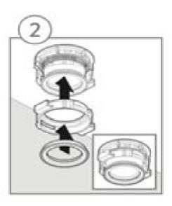
Install mounting assemble on sink
