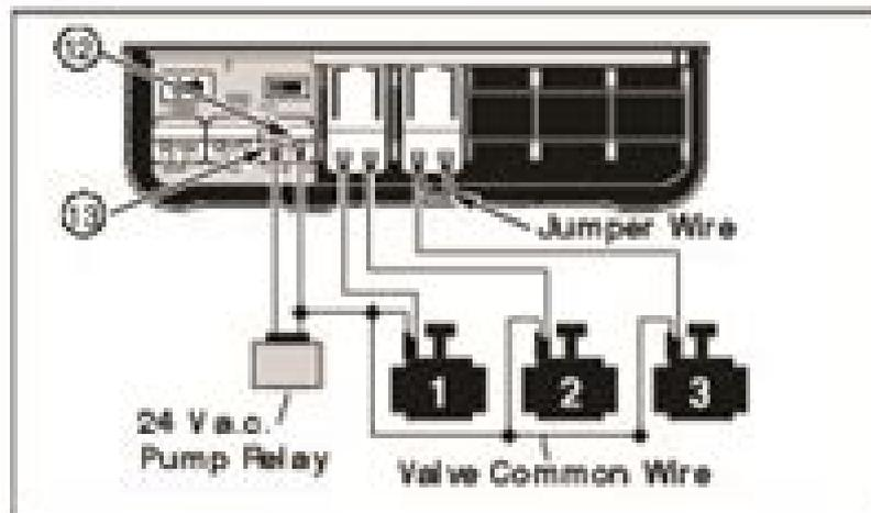
**CAUTION** To prevent pump damage due to "dead heading," connect a jumper wire from any unused zone terminal to a zone terminal with a valve connected.
