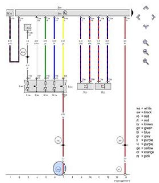
Operating unit in front of centre console, Rear parking aid warning buzzer, Front parking aid warning buzzer, Parking aid control unit, Park assist steering control unit
