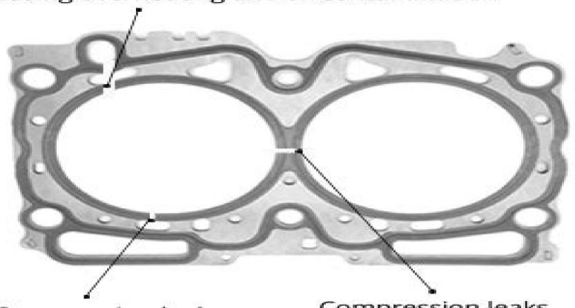
Compression leak into cooling causing overheat Compression leaks between cylinders causing misfire or rough idle
