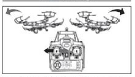
Pull the throttle left or right, the quadcopter turns left or right.
