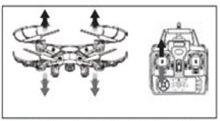
Push the throttle up or down, the quadcopter will ascend or descend.
