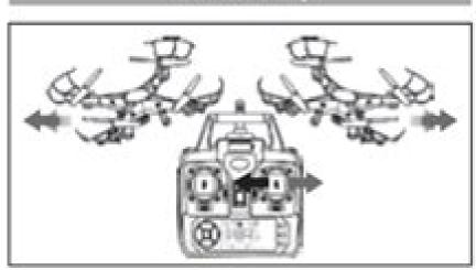
Pull the direction lever left or right, the quadcopter flies to the left side or the right side.
