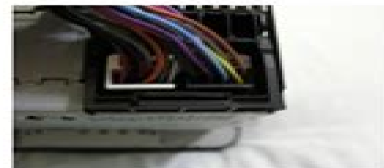
Align and slide the connector into the back of the RNS 510, and close 90 Deg. Clip
