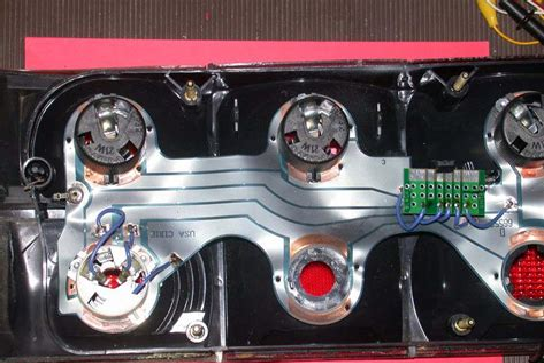
Brake/Tail and harness connector repair
