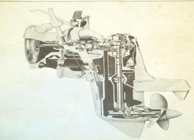
OUTBOARD DRIVE UNIT MODELS B and C
