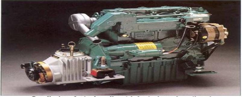
3-cylinder, 4-stroke, direct injected marine diesel with reverse gear, V-drive or S-drive. Propeller shaft output, — 20.5 kW (28 hp) at 3200 r/min.
