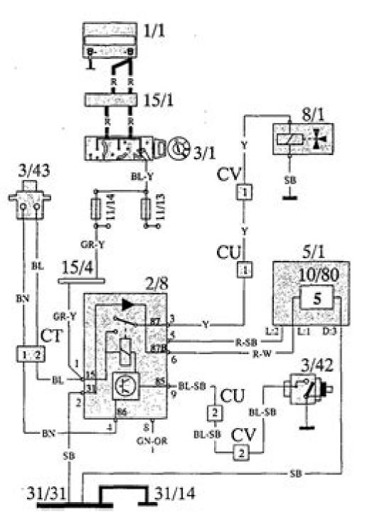
1/1 Battery 2/8 Overdrive relay 3/1 Ignition lock Contact on gearbox 3/42 3/43 Contact in gear lever 5/1D 4-pin connector in combined instrument 5/1L 2-pin connector in combined instrument 8/1 Operating solenoid 10/80 Indicator lamp, overdrive 11/1 - 35Fuses 15/1Positive terminal 15/4 15I-rail in relay unit Ground connector at relay unit 31/14 Ground connector rail in relay unit 31/31 CT Connector at relay unit CU Connector at relay unit CV Connector at gearbox
