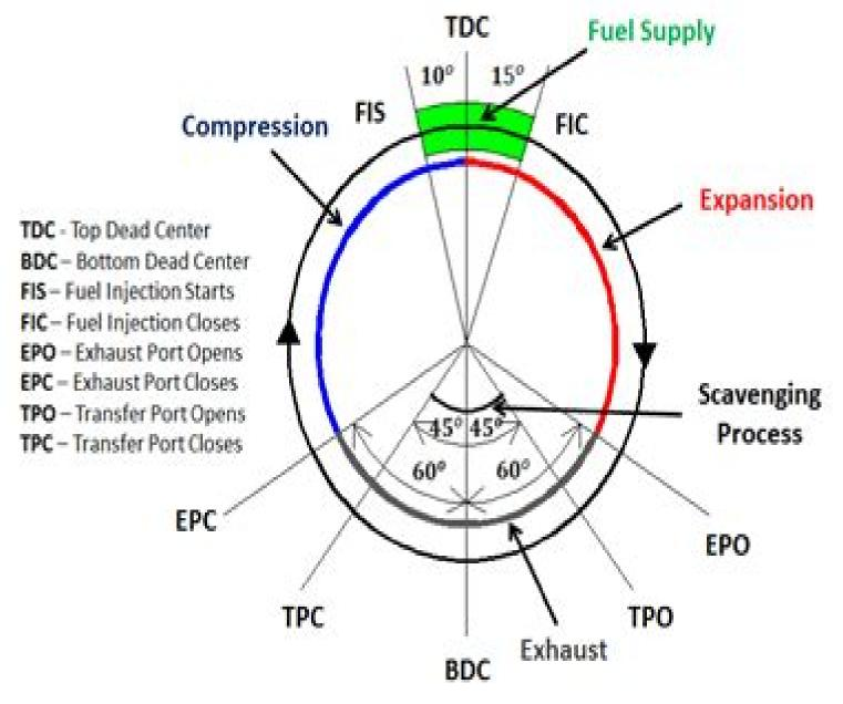
©2017mechanicalbooster.com Valve Timing Diagram of 2 Stroke diesel Engine
