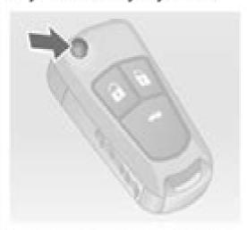
Press button to extend. To fold the key, first press the button.
