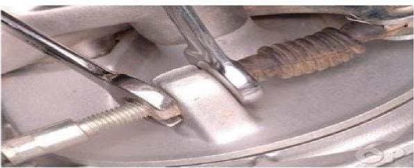
Return the brake adjusting nuts to their original position and check the front brake free play. See the <u>Front Brake Inspection topic</u> for more information.
