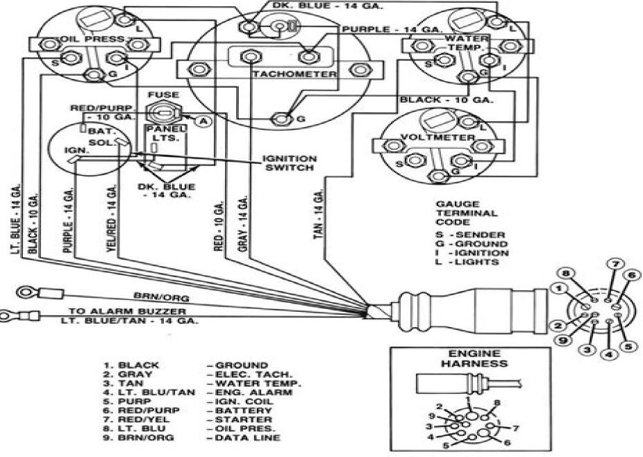
NOTE: ENGINE HARNESS WIRED FOR PANELS USING VOLTMETERS ONLY.
