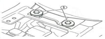
Remove the seat. Remove the two bolts ①.
