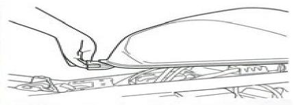
Lift the rear end of the fuel tank and slide it back.
