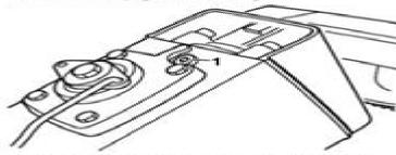
Tilt the stemdrive to the full up position. Remove the fill plug (1) and fill with approx. 2.2 litres of DuraPlus \*\*GL-5 synthetic gear oil. Install the fill plug with a new gasket. Tighten the fill plug to 35 N·m (26 ft. lb.). Lower the stemdrive and check the oil level with the dipstick. If necessary, top off the stemdrive with oil through the dip stick hole.
