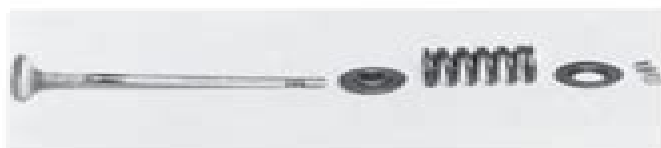
94. Remove the valve locks, retainers, springs, the lower washers (exhaust) and the valves. NOTE! Make sure not to mix the parts!
