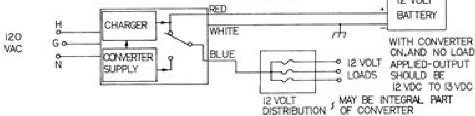
SIMULATE FULLY CHARGED BATTERY ON EITHER UNIT WITH A 50 OHM,10W RESISTOR IN PARALLEL WITH A 50,000 MFD CAPACITOR CONNECTED TO THE CHARGER OUTPUT
