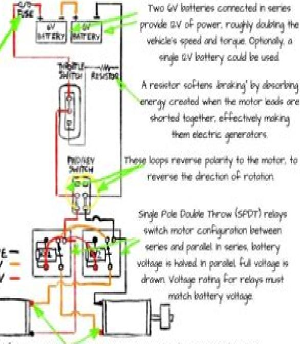
Polarity of motors are reversed from one another, since motors are oriented in apposing directions.
