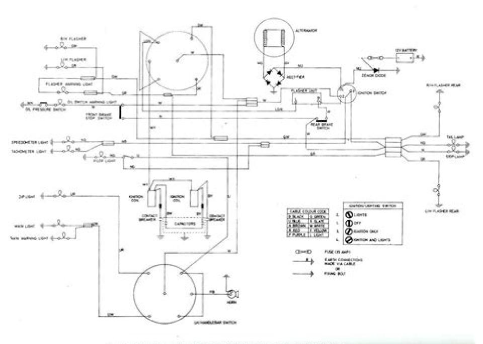
Schematic wiring diagram of a 650cc Triomph 1971 model, up to Engine No. HG36870.
