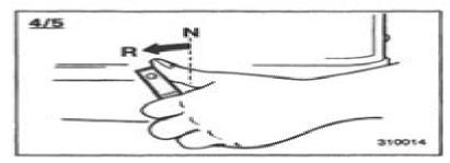
Turn the gear shift lever quickly and firmly from Neutral to Reverse.
