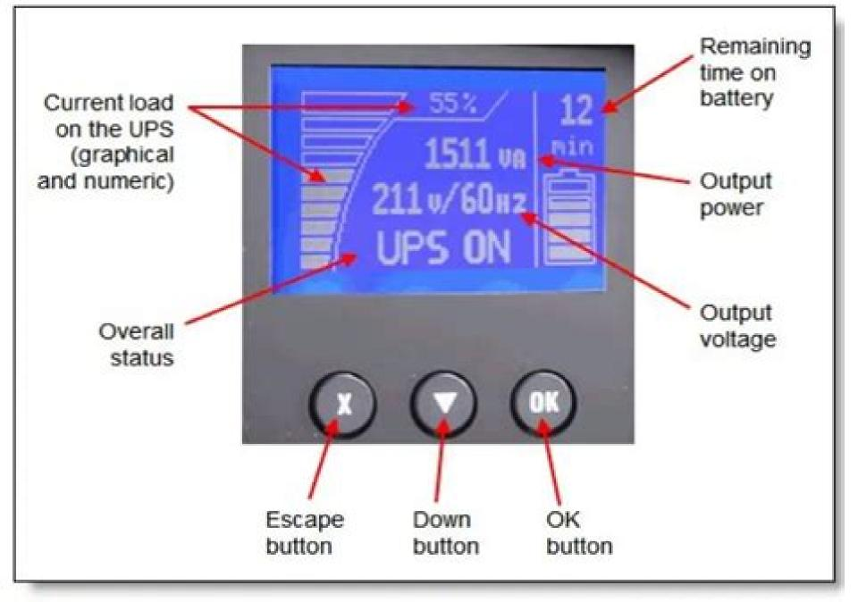
Figure 2. Front panel (showing System Status)
