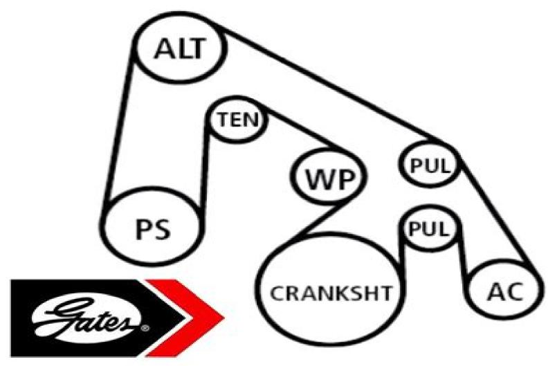
SERPENTINE DRIVE BELT HOLDEN V6 ECOTEC 3.8L MOTOR WITH AIR 1997-01 HOLDEN VT-VX COMMODORE 1999-01 HOLDEN WH STATESMAN 2000-01 HOLDEN VU UTE
