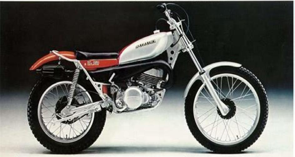
Maximum Murapposer 18.0 Api8,000 rpm S.A.E. NET Maximum Tongue: 2:30 Apim 116.6 In-bi24,500 rpm Engine Type: 2-brooks, single cylinder Paton Displacement: 246 cc (15.0 cu-le) Tonemation: 5-apied, constant mesh fruit Tank Cassoty: 5.0 by (1.3/1.1 US/hmp-pal) Lubritation: Cassot michure Cheryll Length: 2,005 mm (80.1 ini Oserall Blatch: 850 mm (30.5 ini)
