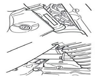
The frame number ① is stamped on the steering head as shown in the illustration. The engine serial number ② is stamped on the crankcase assembly.
