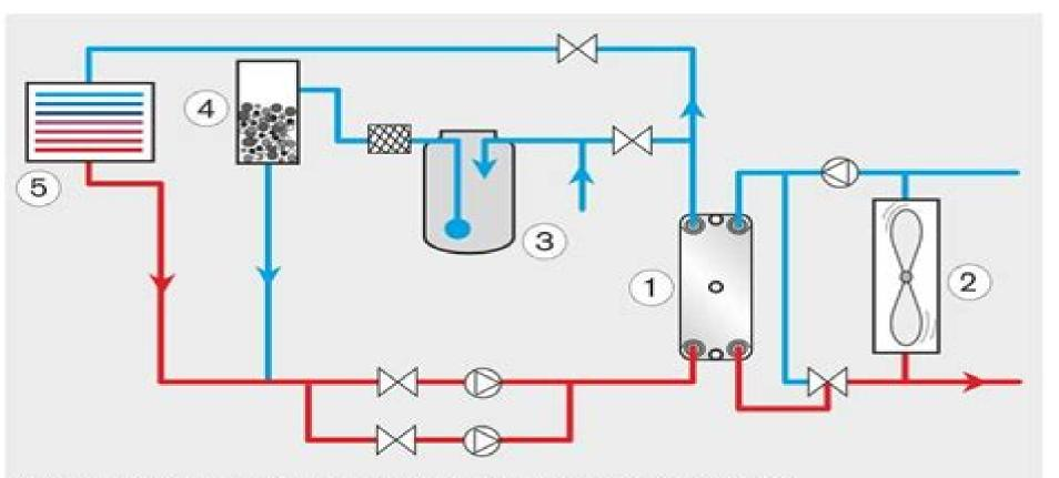
The treatment circuit with an ion exchanger (4), fine mechanical filter, air removal facilities and an expansion tank (3) keep the water deionised.
