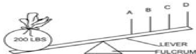
Q. In the preceding diagram, it would be easiest to lift the weight by applying pressure at point:
