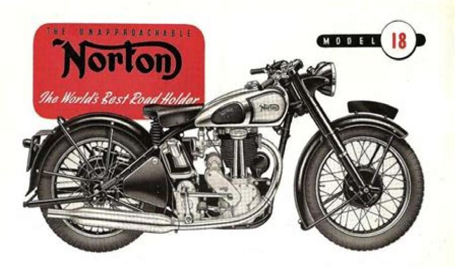
THE MODEL 18 ENGINE employs overhead valves, push rod operated; the whole of the valve gear is totally enclosed and automatically lubricated. Positive lubrication large bearing surfaces and ground timing gear toeth ensure silent operation. The engine has a lone and stroke of 79 m.m. x 100 m.m. and a subic capacity of 490 c.c.
