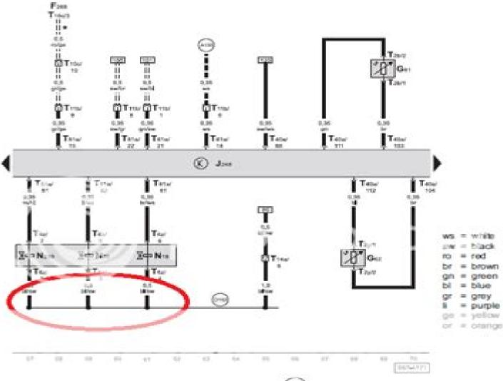
F268 - Heater element contact switch (PTC)
