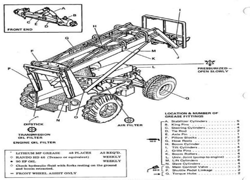
Figure 1. Lubricating and Maintenance Points
