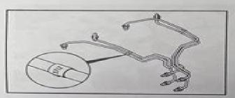
Caution: Do not weld or substitute lines; use only the specified part number for the engine.
