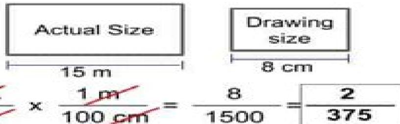
The scale factor is  $\frac{2}{375}$  which means that the drawing size is  $\frac{2}{375}$  times the actual size of the garden.
