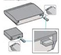
Connect the AC power cords of the main unit, surround amplifier, and your TV to the AC power outlet, and then turn on the power of the main unit and your TV.
