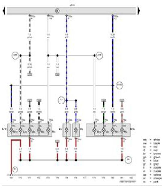
Onboard supply control unit, Left tail light, Right tail light, Left number plate light, Right number plate light.
