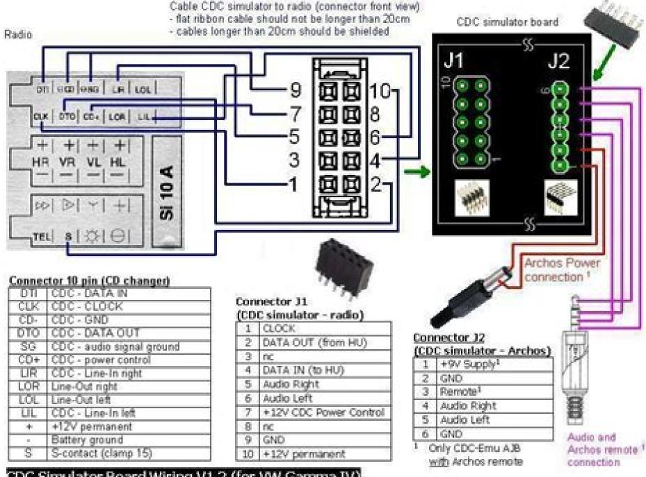
CDC Simulator Board Wiring V1.2 (for VW Gamma IV)
