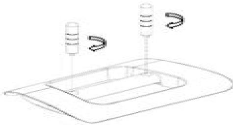
Load the two holders and the stand together, and make sure they are secure and tie.
