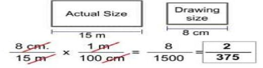
The scale factor is 2/375 which means that the drawing size is 2/375 times the actual size of the garden.
