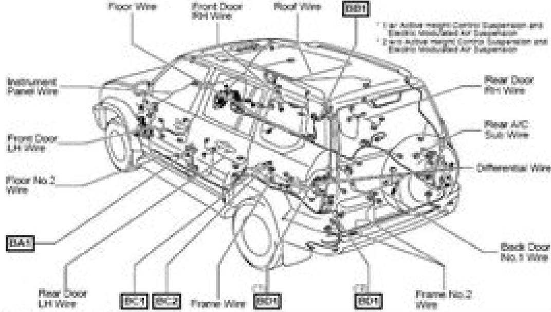
\* 1 for Active Height Control Suspension and Electric Includable Air Suspension
