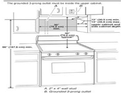
"30" (76.2 cm) is typical for 66" (167.6 cm) installation height. Exact dimensions may vary depending on type of range/cooleop below.
