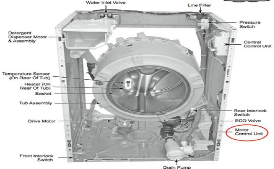
Not Shown: Console, Touchpad/LED Assembly, & Door Switch Assembly
